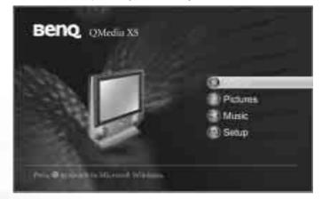
The usual way of tapping on the touchpad to make a selection does not work under QMedia XS mode, you have to press the touchpad selector button to effect a selection.
